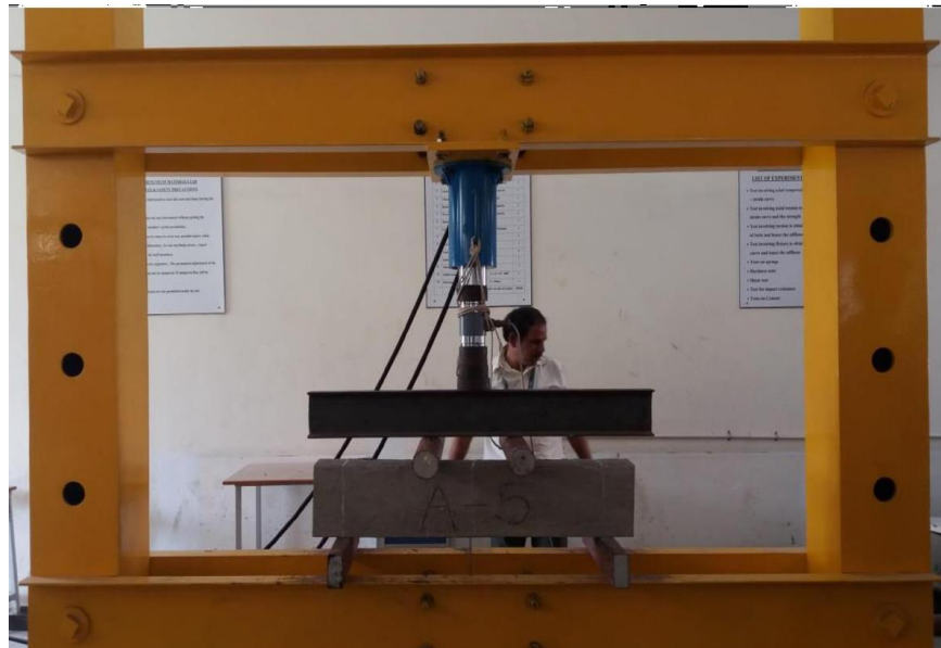
Fig.4: Flexural Strength Test Arrangement.
